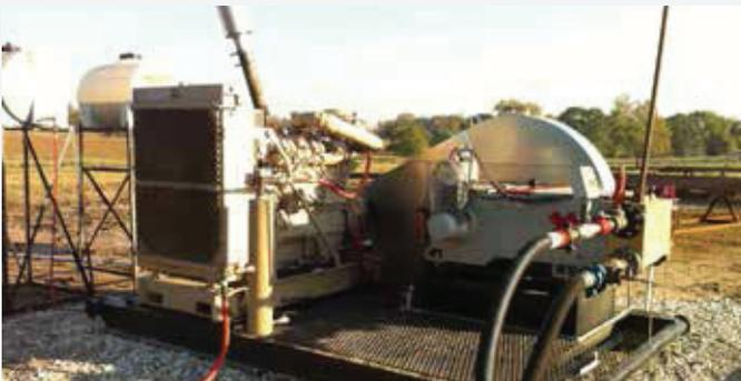
Permanent unit with Cummins natural gas engine.
